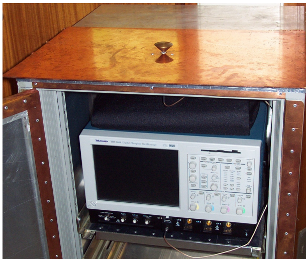
Figure 7. View of the Faraday cage with the biconical antenna mounted.
